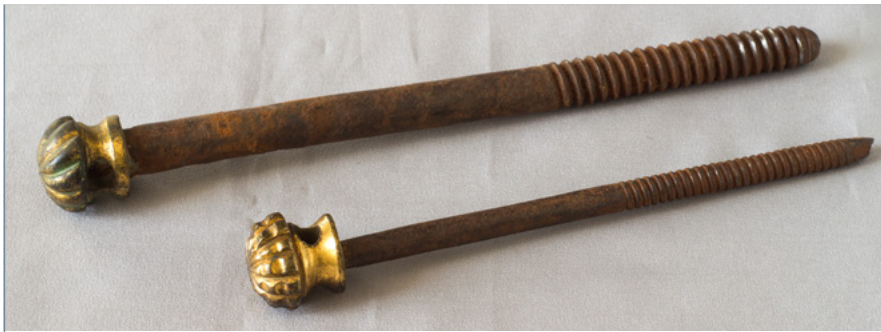
[fig. 33] Iron-alloy arming bolts with gilt copper-alloy heads.
